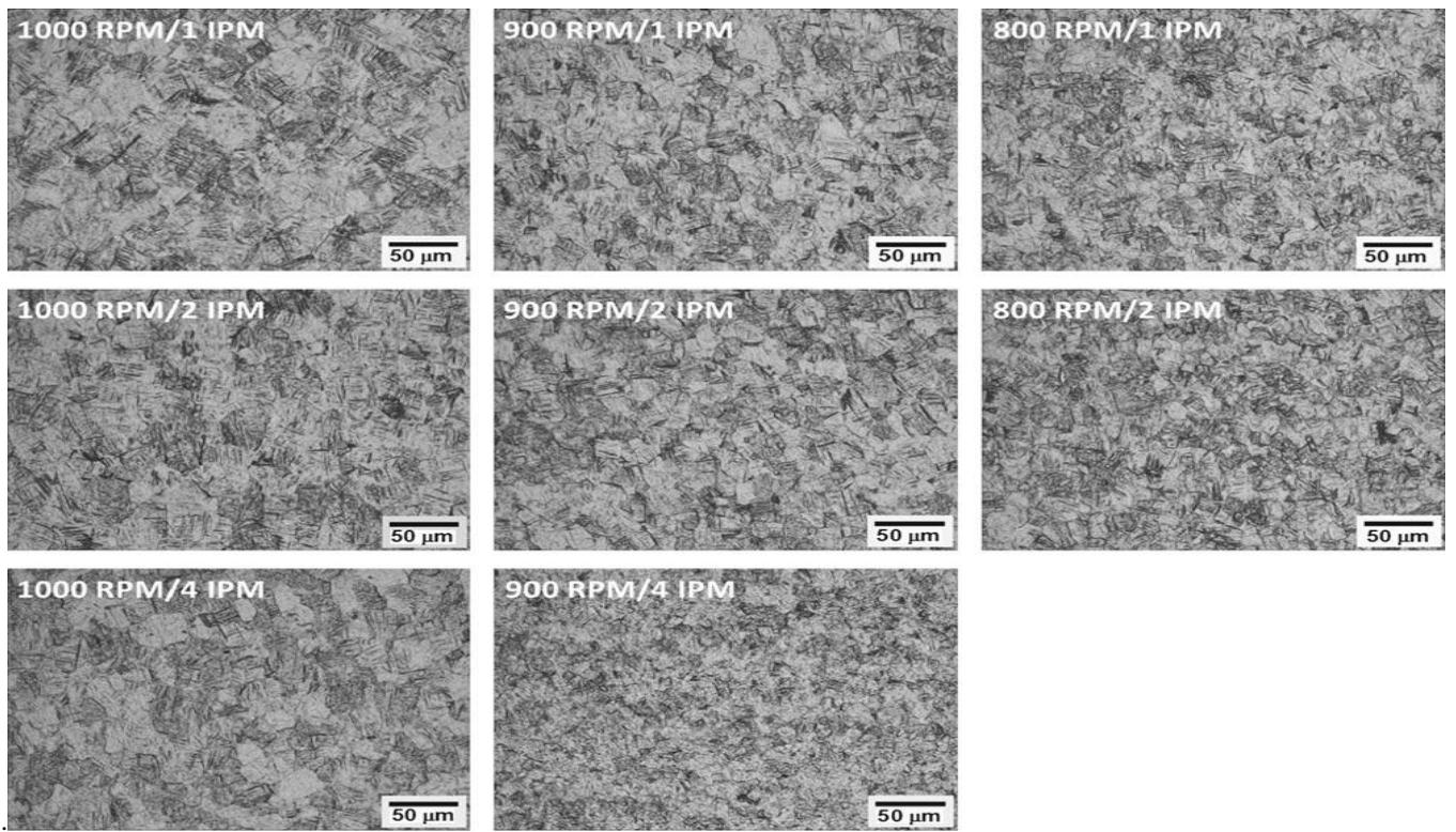
Figure 3: Optical micrographs taken from center of the SZ in the samples with different processing parameters [6].
