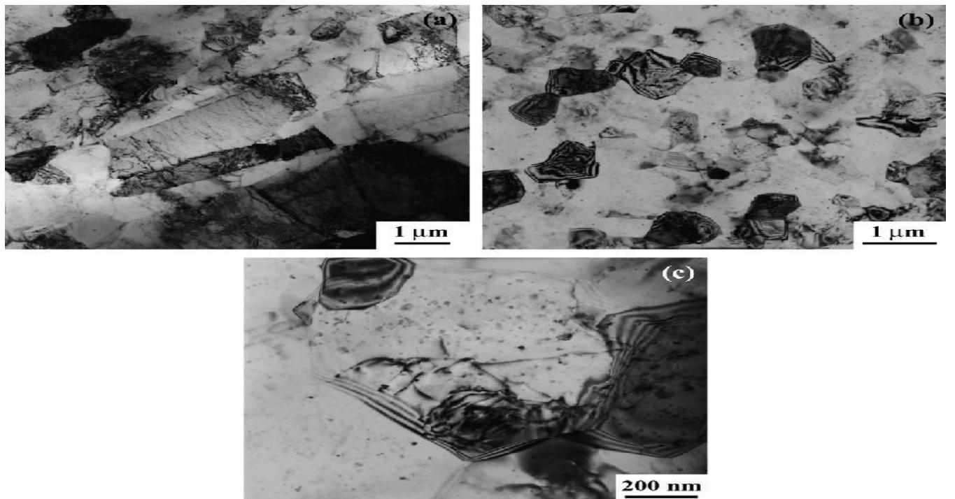
Figure 4: TEM images showing grain structure and dispersoid distribution in (a) as-extruded Al-Mg-IZr, (b) & (c) FSP Al-Mg-IZr [7]
