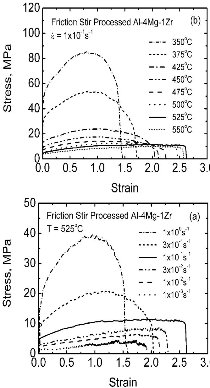
Figure 10: Stress strain behavior of friction stir processing Al-4Mg-1Zr, (a) initial strain rate at  $525^\circ\text{C}$ , (b) temperature at an initial strain rate  $1 \times 10^{-1} \text{ s}^{-1}$  [33]
