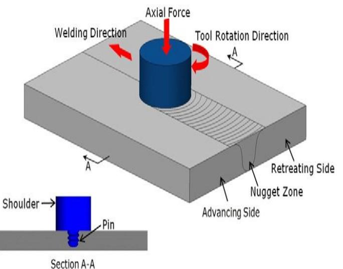
Figure 1: Friction Stir welding
