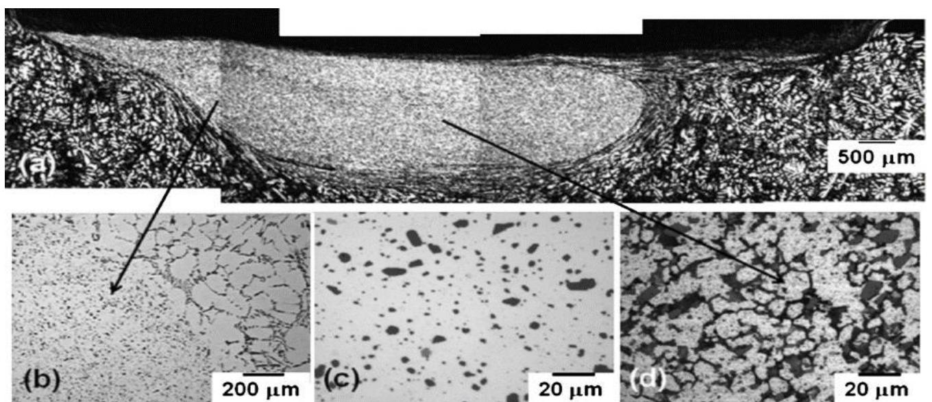
Figure 8: (a) Cross-section optical macrograph of a single pass run, (b) interface between cast and FSPed region showing extent of particle refinement, (c) higher magnification image shows size and shape of Si particles inside the FSPed nugget and (d) grain structure inside the nugget [22]
