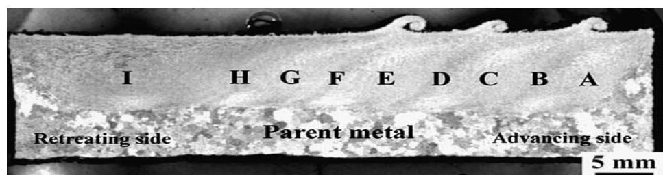
Figure 5: Macrographs showing nugget and transitional zones of 5-pass FSP A356 [13]
