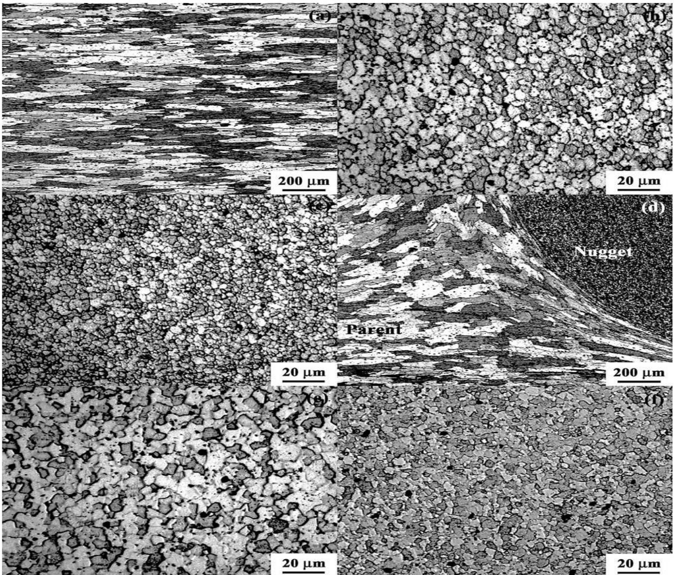
Figure 9: Optical micrographs showing grain structure of (a) parent zone, (b) FSP zone, 4 ipm/400 rpm, (c) FSP zone, 6 ipm/350 rpm, (d) transition zone, 4 ipm/400 rpm, (e) FSP zone, 4 ipm/400 rpm after heat treatment at 490 °C/1 h, and (f) FSP zone, 6 ipm/350 rpm after heat treatment at 490 °C/1 h [23]
