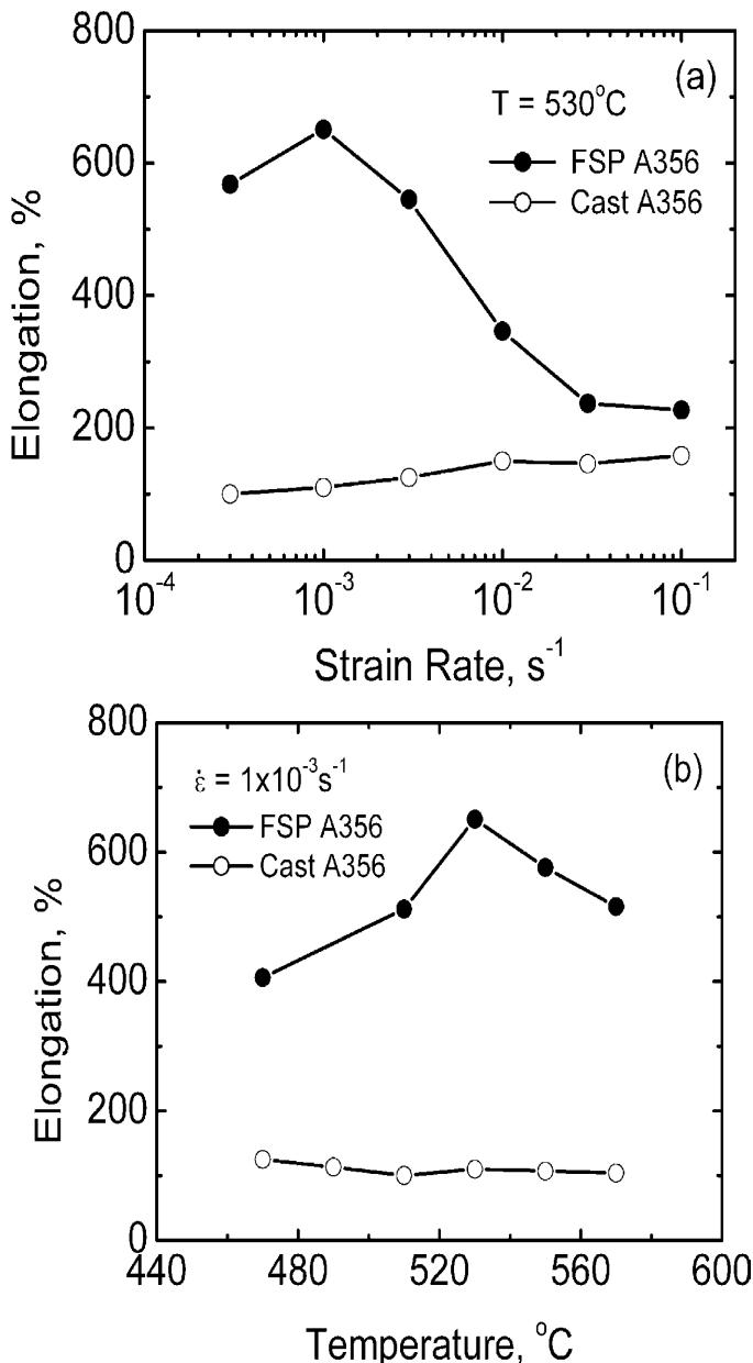
Figure 12. Variation of elongation with (a) initial strain rate and (b) temperature for both FSP and cast A356 [34].
