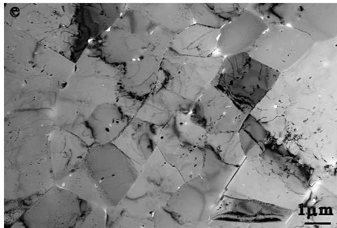
Figure 7: Grain structure in different weld regions: (a) base metal, (b) dark field image of region (a), (c) HAZ, (d) TMAZ I, (e) TMAZ [21]
