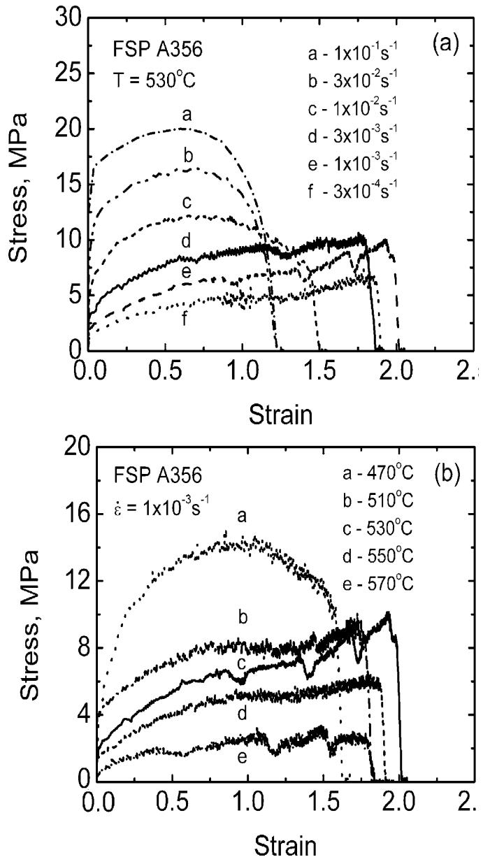
Figure 11: Stress-strain behavior of FSP A356 as a function of (a) initial strain rate at  $530^\circ\text{C}$  and (b) temperature at an initial strain rate of  $1 \times 10^{-3} \text{ s}^{-1}$  [34]
