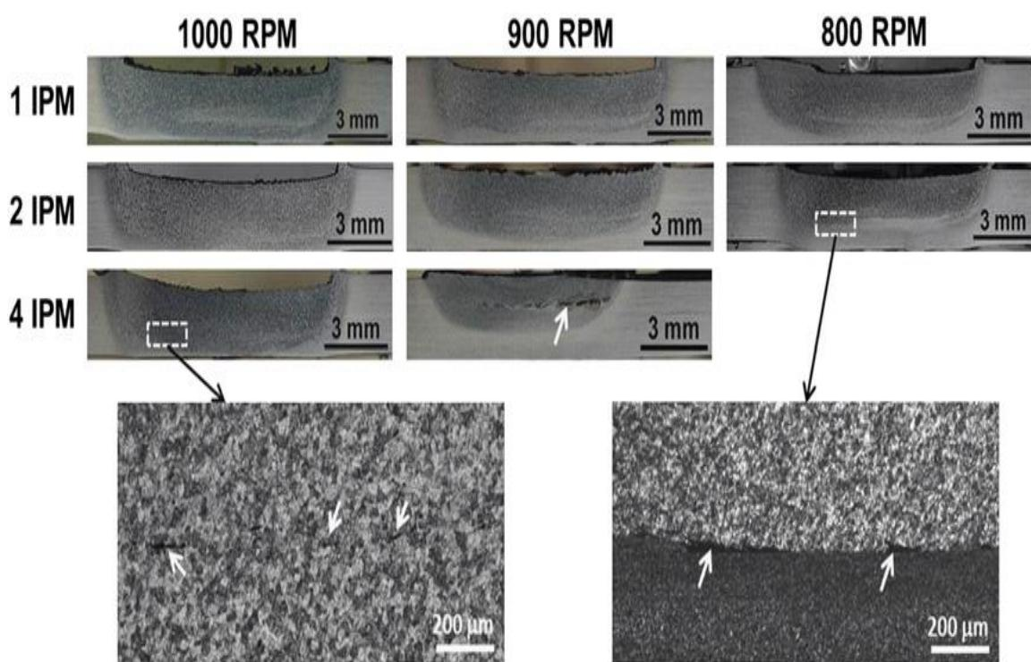
Figure. 2. Cross-section macrographs of FSP Ti–6Al–4V samples processed at different combinations of tool rotational speed (RPM) and tool traverse speed (IPM). Note that the processing defects are marked by white arrows [6].
