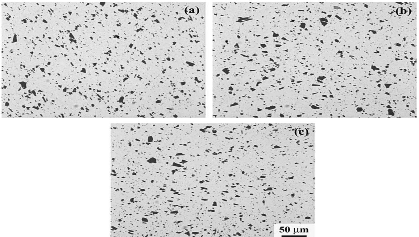
Figure 6. Typical optical micrographs showing Si particle distribution in 5-pass FSP A356: (a) 1st pass, (b) 2nd–3rd pass transition, and (c) 5th pass (locations A, D, and I in Fig. 5) [13]
